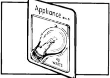
Remove the light bulb from its socket. Replace the bulb with a 40-watt appliance bulb.
