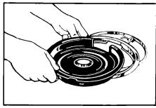
2. Line up openings in the reflector bowl and notches in the trim ring with the surface unit receptacle and the element hold down clip.
