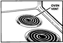
The vent is needed for air circulation. **Do not block the vent.** Poor baking can result.
