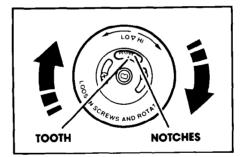
**4.** To raise the temperature, move the tooth a notch closer to HI. Each notch equals about 10°F (5°C).
