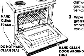
4. If you want the oven racks to remain shiny, remove from the oven and clean by hand. Otherwise, put oven racks on second and fourth guides (guides are counted from bottom to top). After racks are cleaned in the Self-Cleaning cycle, they become harder to slide. Apply a small amount of vegetable oil to the sides of the racks to make them easier to slide. See chart on page 22.
