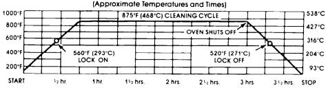
Notice that the heating stops when the 3-hour setting is up, but that it takes longer for the oven to cool down enough to unlock.
