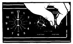
**4.** Push in and turn the Stop Time Knob **clockwise** to the time you want the oven to shut off.
